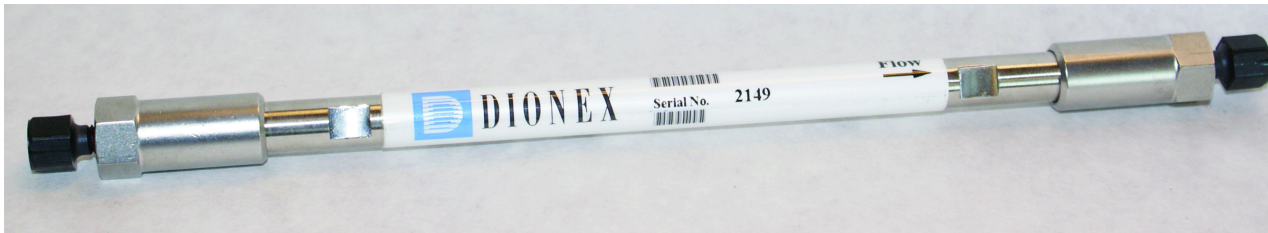
HPLC steel column (internal diameter 4.6 mm, length 150 mm)
